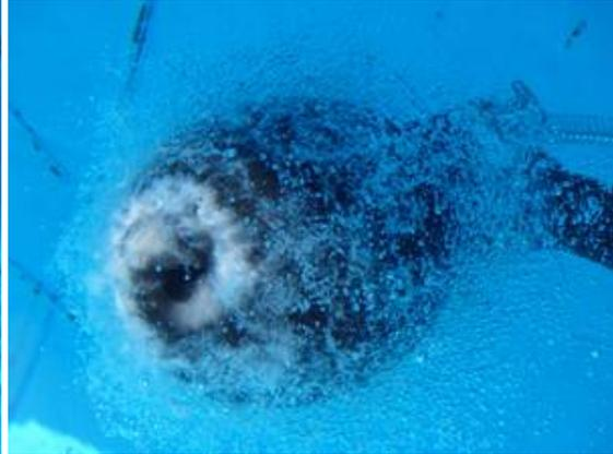
A close up on the system during action in a pool showing the fine bubbles leaving the units.
